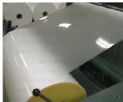
High-speed processing generates electrostatic charging as a result of the sudden separation of the foil surfaces
