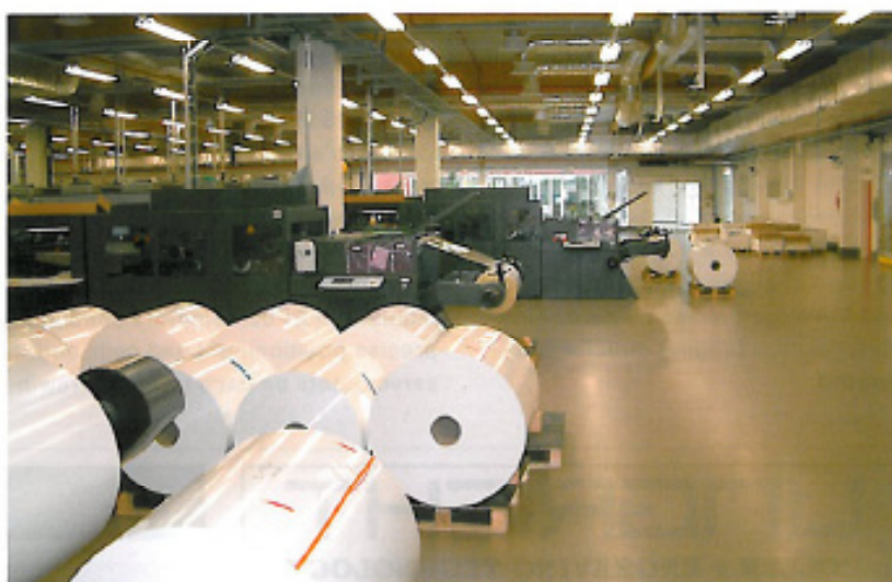
Synthetic polypropylene film have a sensitive reaction if the humidity is too low
